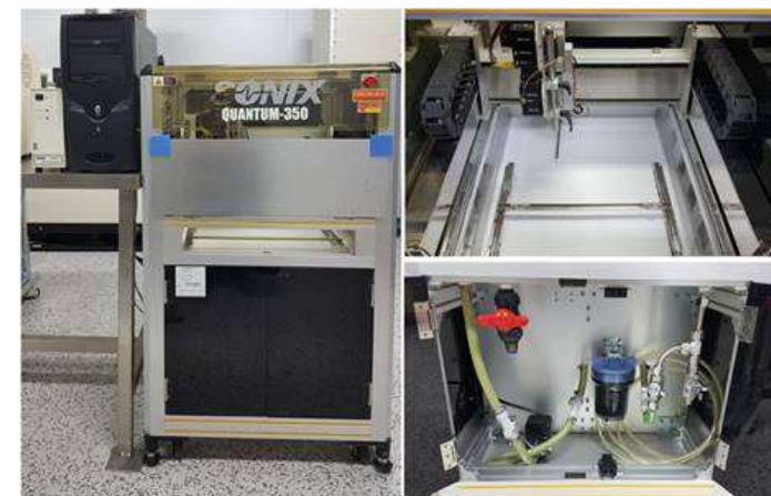
C-SAM: Sonix Quantum 350H Spatial resolution: 0.5 \mu m Depth resolution: 8 \mu m
